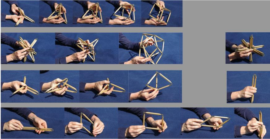
**Fig. 5.** Top: folding down the hull. Hull in centre, bundles left and right; 1st row: cube—the hull of tetrahedron and tetrahedron; 2nd row: rhombic dodecahedron—the hull of cube and octahedron; third row: hull of “triangular dipole and triangular cushion”; 4th row: hull of “duogonal dipole and dougonal cushion” (for row 3, 4 compare paragraph 3.1: polyliner with duogon)
