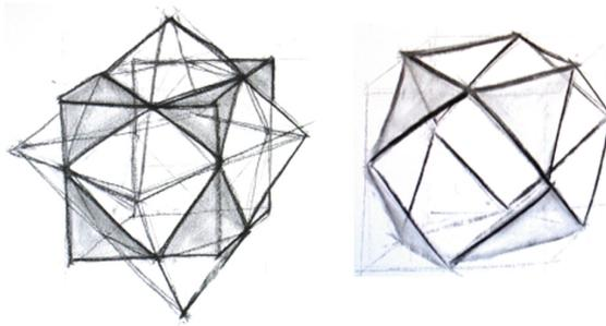
**Fig. 3.** Intersection—mid-point of transformation process. Left: cube and octahedron in a relative size so that all their edges meet in pairs; right: kernel—their shared volume: the cubeoctahedron
