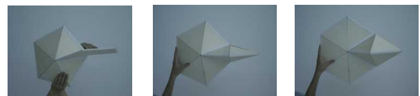
Figure 2: Deformation of the Goldberg icosahedron (Fig 1, right). Left: in one extreme position: the right unit is completely flat. Centre: in the neutral position, both units have the same shape. Right: in the second extreme position, the left unit is completely flat.
